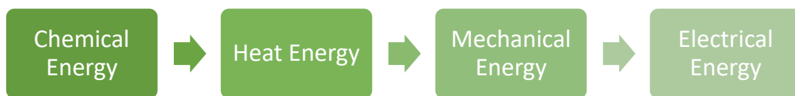
Figure 21: Energy conversion in Diesel Engine based Gensets
